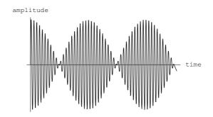
Figure 1.1: Sum of two sine waves with frequencies in the ratio 1:1.05.
